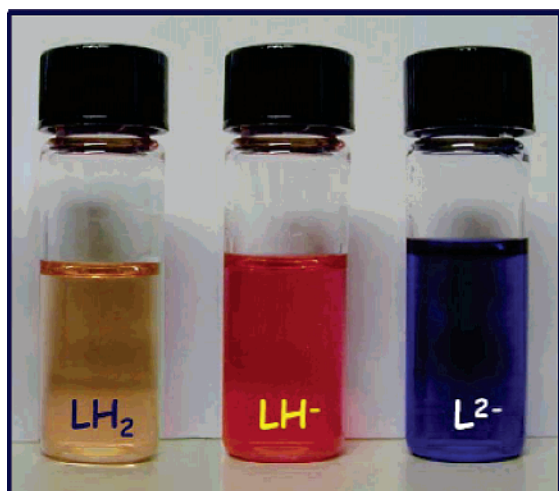
FIGURE 15. Color changes observed on addition of [\text{Bu}_4\text{N}]\text{F} to a DMSO solution of receptor 6 ( = \text{LH}_2 ). From the left-hand: no addition (species present, \text{LH}_2 ); plus 5 equiv of [\text{Bu}_4\text{N}]\text{F} (dominant species, \text{LH}^- ); and plus 40 equiv of [\text{Bu}_4\text{N}]\text{F} (dominant species, \text{L}^{2-} ).
